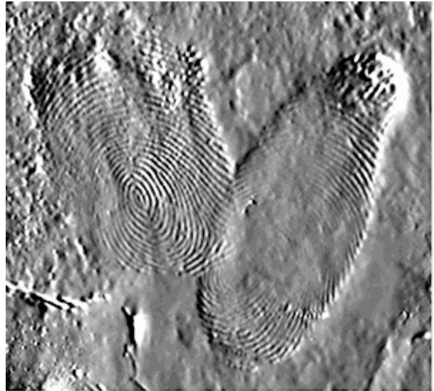
Figure 6. A fingerprint taken from a PTFE insulating plate using an EPIC sensor
